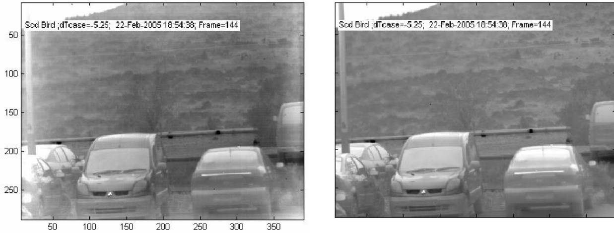
Figure 10: BIRD imagery (50mm lens) illustrating the real-time ambient compensation (right image) after 5.25c drift during 90 minutes with no shutter activation.
